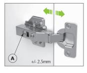
**Depth adjustment** Acting on the "A" screw it is possible to adjust the distance between the side of the cabinet and the door.
