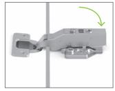
2 Rotate the arm of the hinge.
