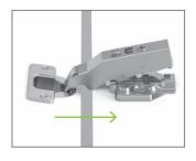
1 Place the front part of the hinge on the front side of the mounting plate.
