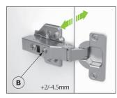
Independent side adjustment Acting on the "B" screw it is possible to change the amount of the door covering on the side of the cabinet.
