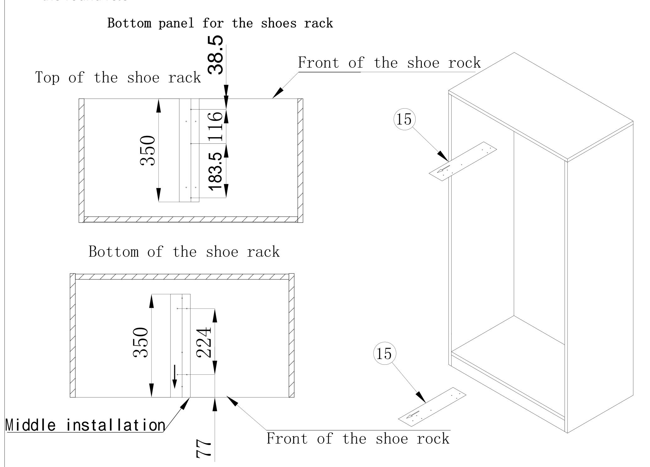
1. 2 Take out 1:1 mounting board, place the lower rail set 4, align the mounting holes drawn in step 1, and install the lower rail set 4 under the bottom panel with four screws 10
